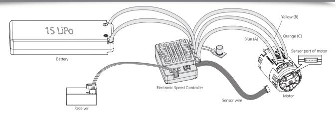
This is an extremely powerful brushless motor system. For your safety and the safety of those around you, we strongly recommend removing the pinion gear attached to the motor before performing calibration and programming functions with this system. It is also advisable to keep the wheels in the air when you turn on the ESC.
